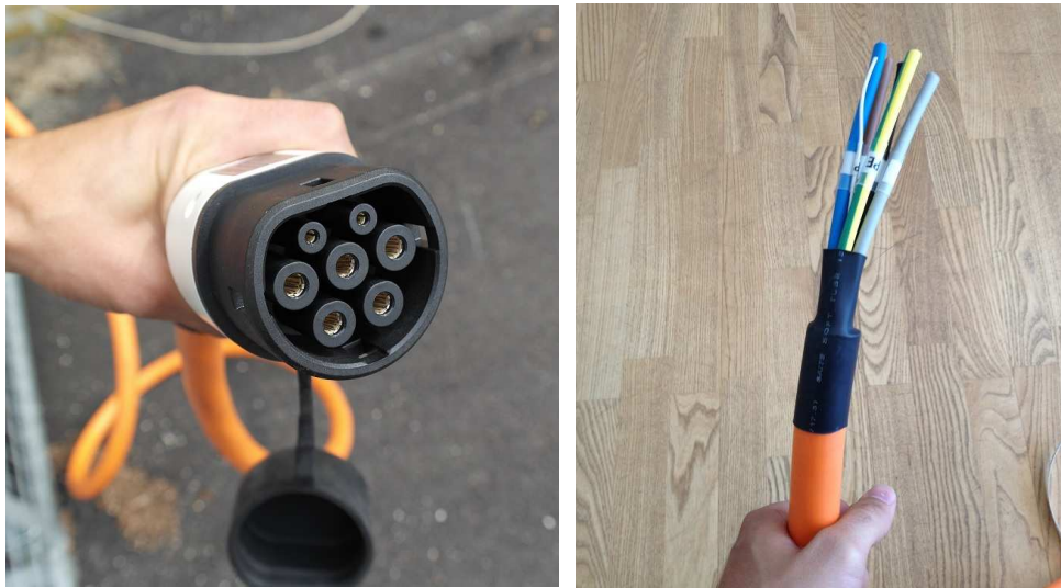
(a) Type 2 63A AC plug. Note three phases, neutral, earth, CP and PP (b) Other end of cable to be mounted in EVSE. The CP wire is also seen.
