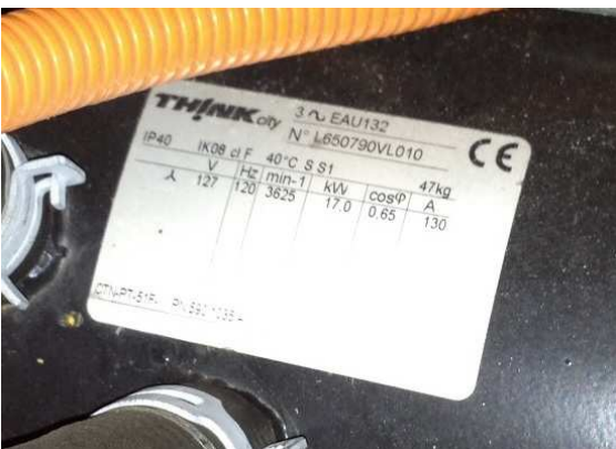
(e) Motor ratings as shown on sticker. 127V wye, 120Hz, 130A, totaling 17kW.
