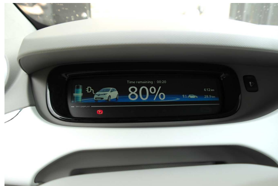
(d) Now showing 80% SOC, 20 minutes remaining: 14% charge in five minutes.
