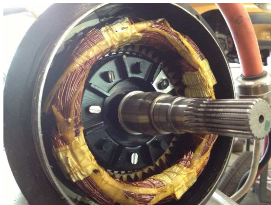
(f) A look inside the motor. The rotor must be held in place by the gearbox, and it is thus easiest to have it mounted in the EV.
