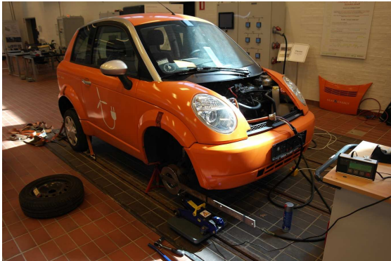
(a) Setup with Think City EV. Torque measurement lever is mounted on right front wheel.
