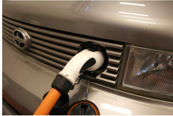
(b) Type 2 connector fits new eBox inlet
