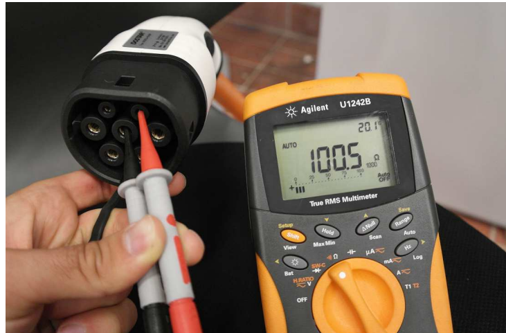
Figure 3.3: Measurement of the PP resistor. 100\Omega corresponds to 63A rating.
