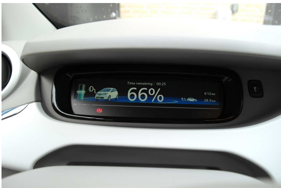
(c) Dashboard showing 66% SOC, 25 minutes remaining.
