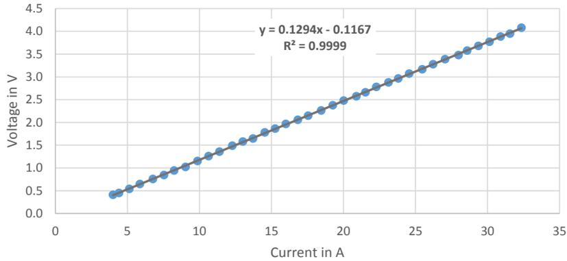
**Figure B.2:** Line-line DC voltage-current characteristic from amplifier
