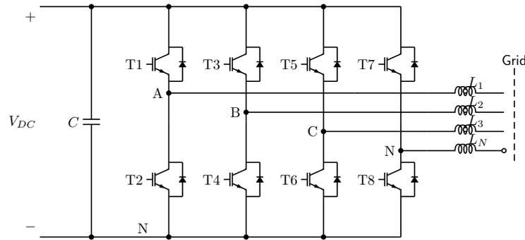
**Figure 2.28:** Three phase four-wire grid connected converter
