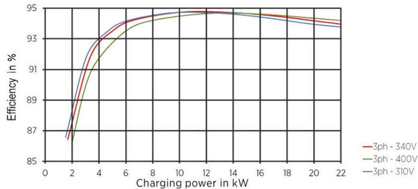
**Figure 2.23:** Efficiency curve of Brusa 22kW charger
