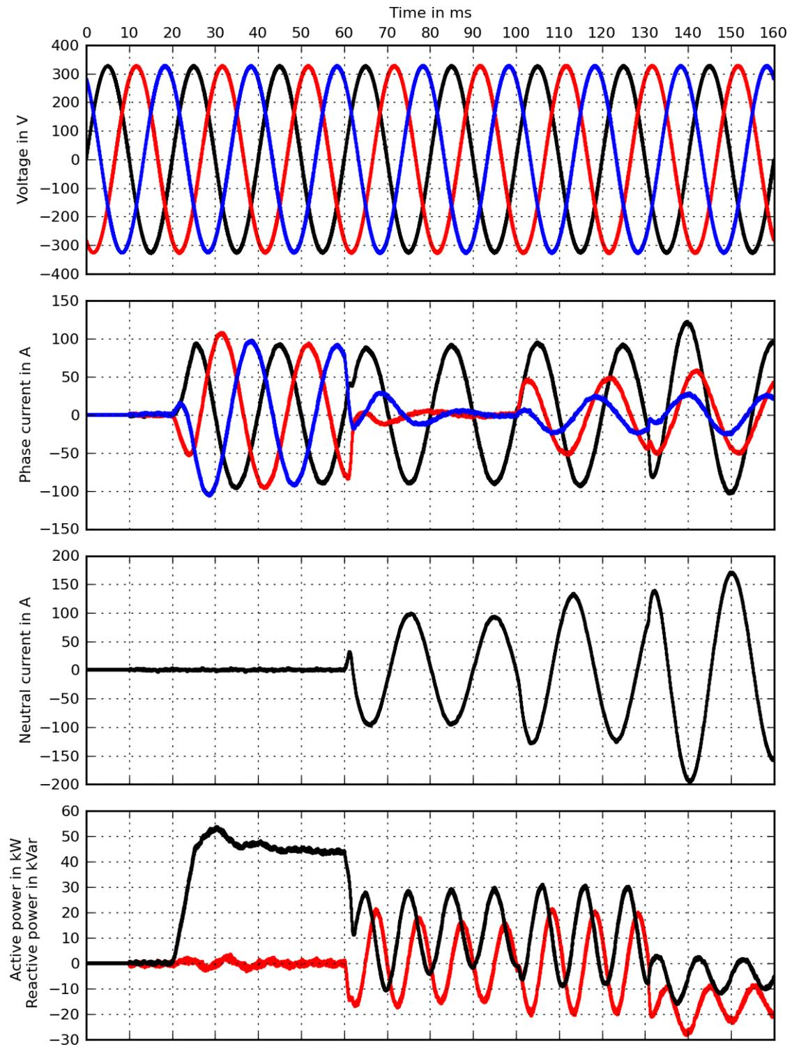
Figure 2.43: Simulation 3 with four-leg converter and per-phase current control
