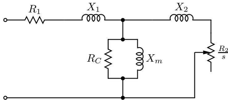
**Figure 2.13:** Induction motor equivalent circuit diagram
