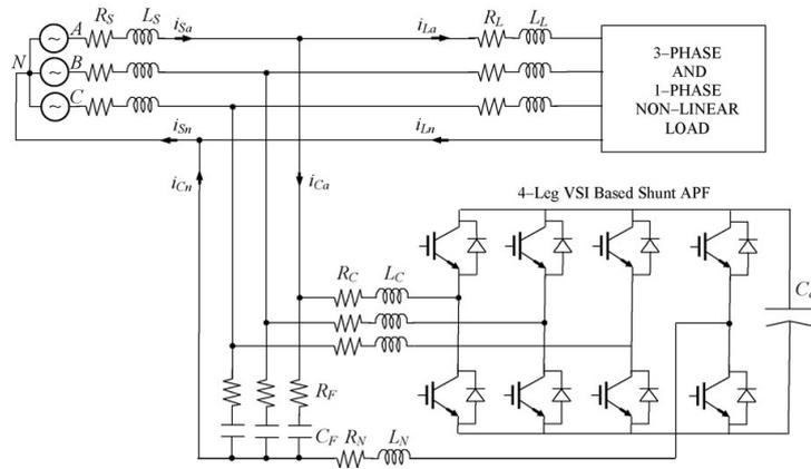
Figure 2.29: Active power filter topology [65]
