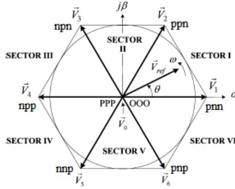
**Figure 2.24:** Switch states drawn in two-dimensional plane [71]
