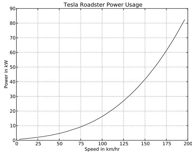
**Figure 1.2:** Tesla Roadster power versus speed [64]
