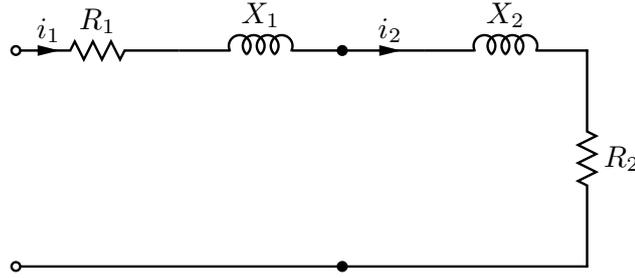
Figure B.3: IM equivalent circuit in blocked rotor test
