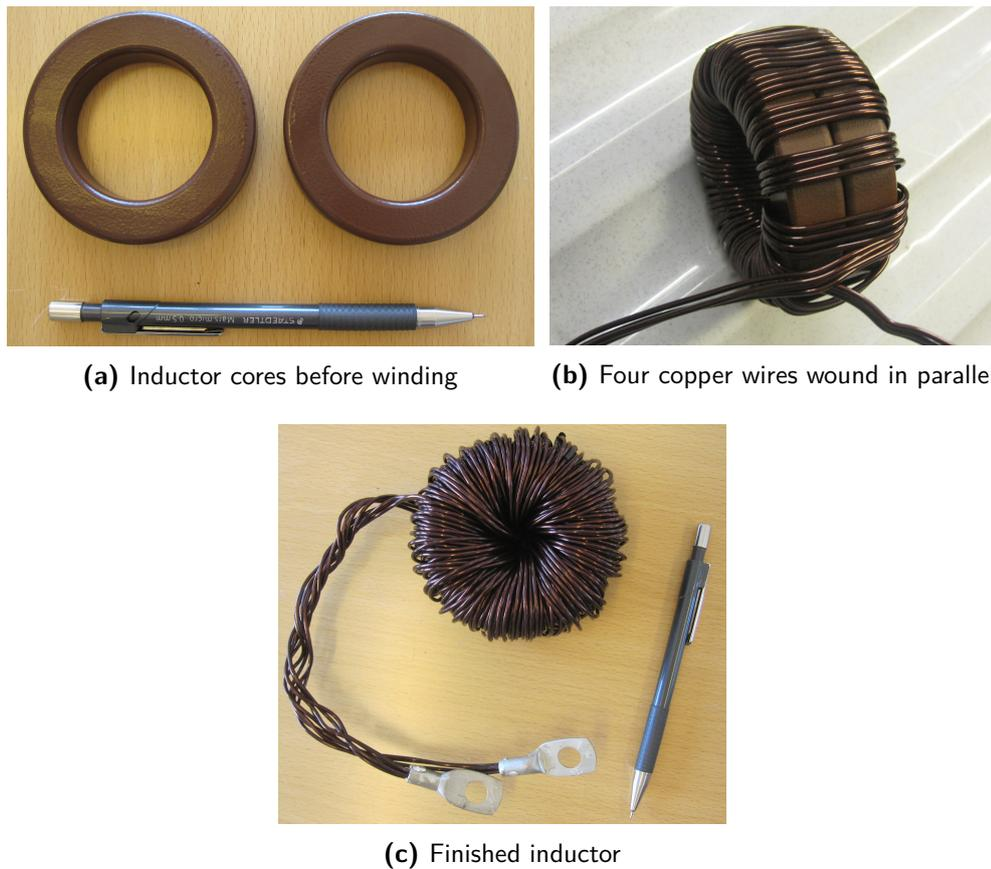
**Figure 2.18:** Inductor prototype
