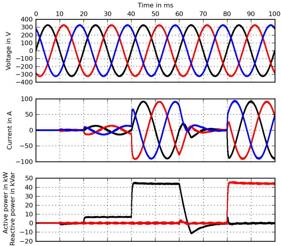
Figure 2.38: Simulation one with balanced grid and three-phase charging
