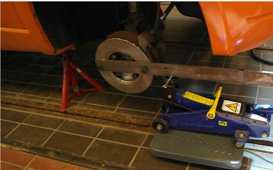
(c) Torque lever mounted on reversed disc brake. It presses on digital scale 20cm from wheel center.
