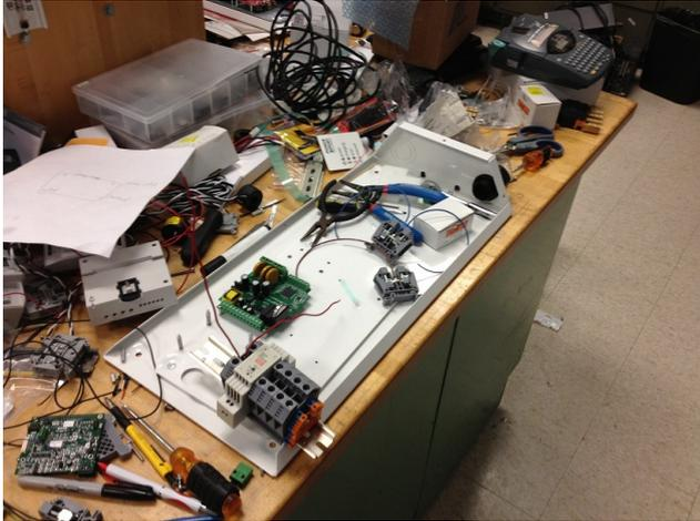
(a) Initial work on three-phase EVSE. It required modifications to all line power components, the power supply and metering, for three-phase capability.
