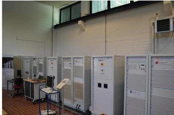
(d) Three-phase 150kW power amplifier connected to the motor. The cable to the motor is quite long and must be taken into account.
