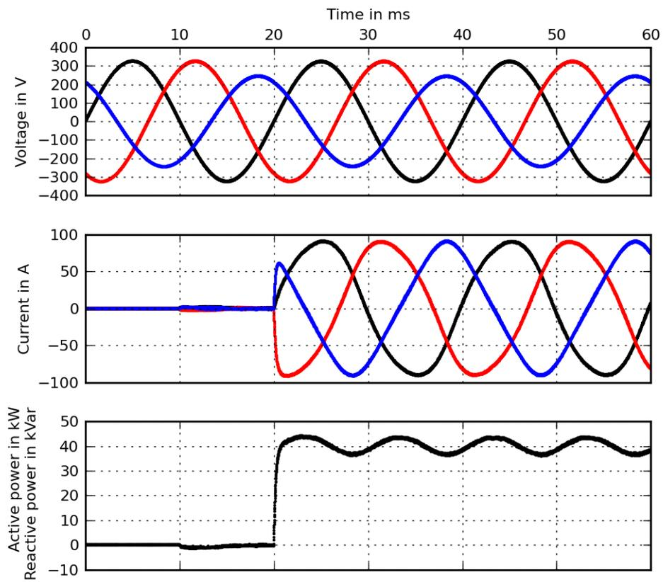
**Figure 2.40:** Simulation 1 with unbalanced grid. Note the distortion of the current, which increases THD
