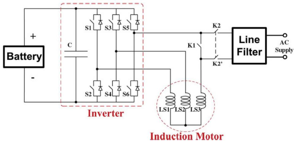
Figure 2.16: AC Propulsion single-phase topology, from [39]
