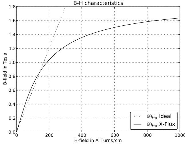
**Figure 2.17:** B-H curve for the chosen inductor core
