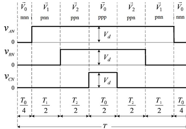
Figure 2.37: Segment determination for each switching cycle in sector 1 [71]
