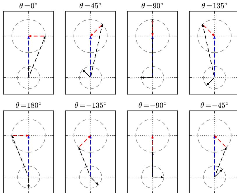
Figure 2.12: Multiple phasors with varying power factor angle
