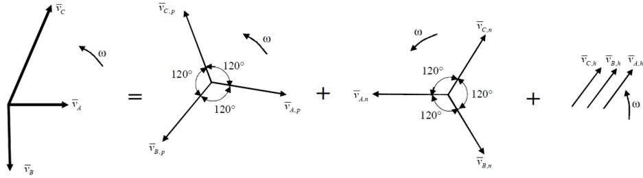
**Figure 2.26:** Any unbalanced voltage can be decomposed into positive, negative and homopolar components [66]
