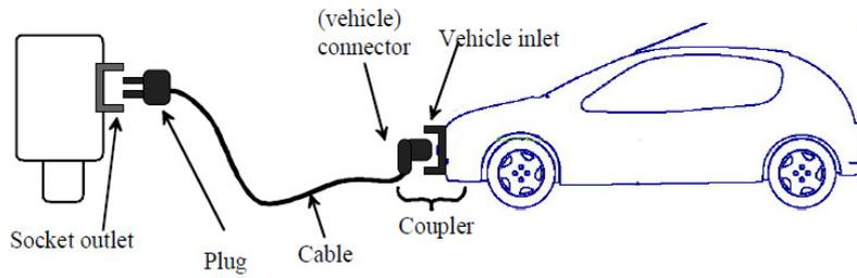
**Figure 3.1:** Cord set terminology according to IEC 61851-1 [5]
