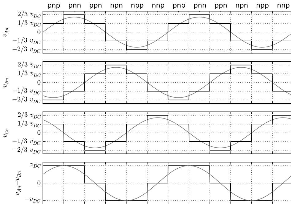
Figure 2.4: Switching scheme for generating three-phase voltages
