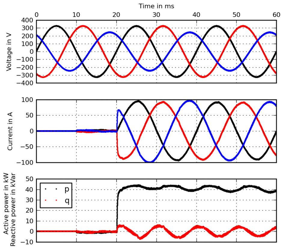
**Figure 2.42:** Simulation 2 with unbalanced grid. Note the currents are balanced and sinusoidal
