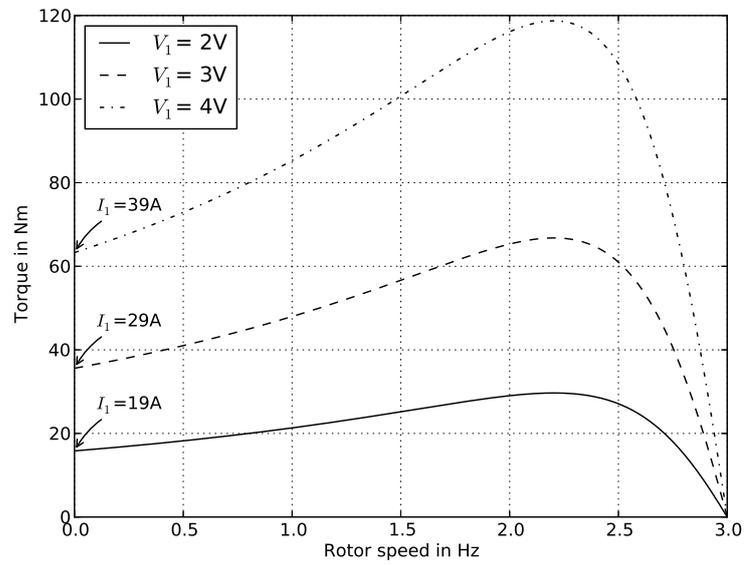
Figure B.14: Torque versus current at 3Hz supply frequency
