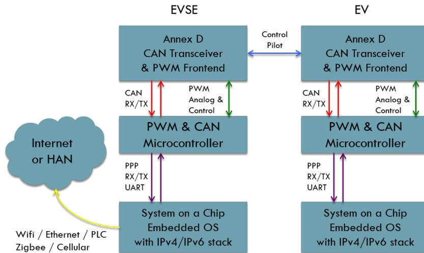
**Figure 3.7:** System level diagram of Annex D implementation
