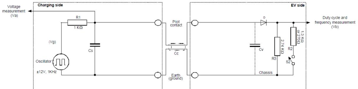
**Figure 3.4:** Typical pilot function schematic [5]
