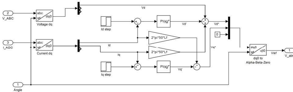
Figure 2.33: Single  $dq$  controller implemented in Simulink
