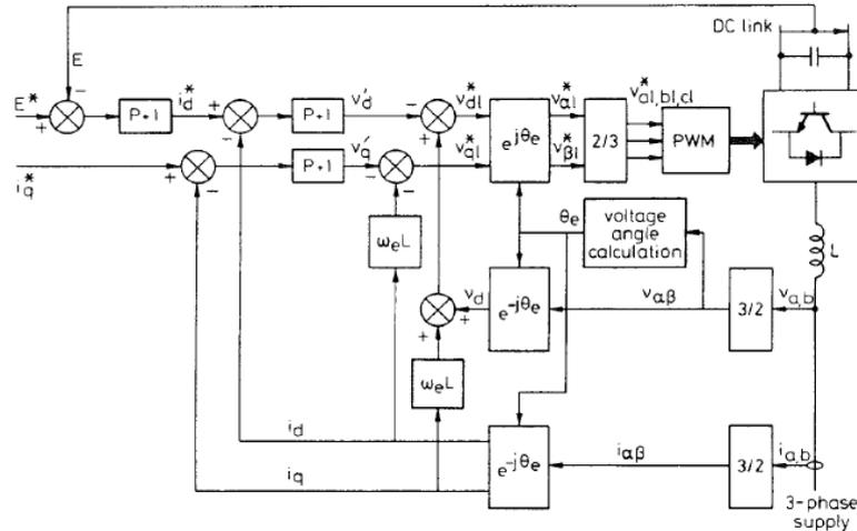
**Figure 2.25:** Three-phase converter control using  $dq$  transform [61]
