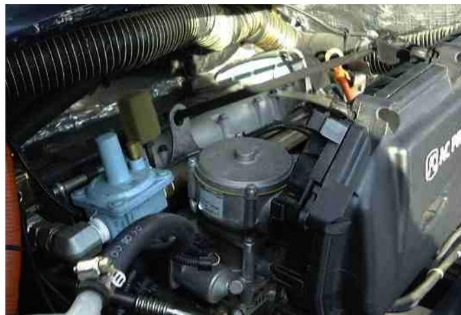
**Figure 8. Natural Gas Fuel System Components**
