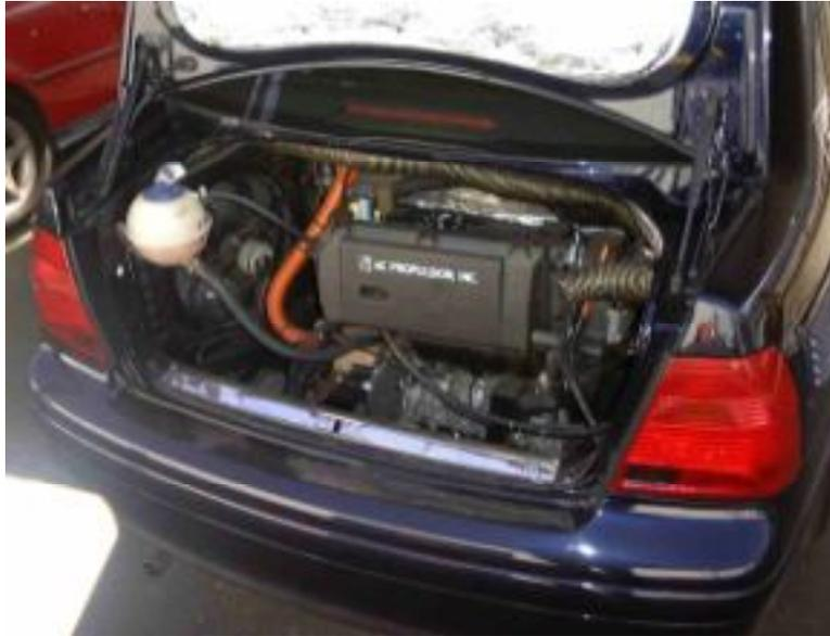
**Figure 7. APU Installed**
