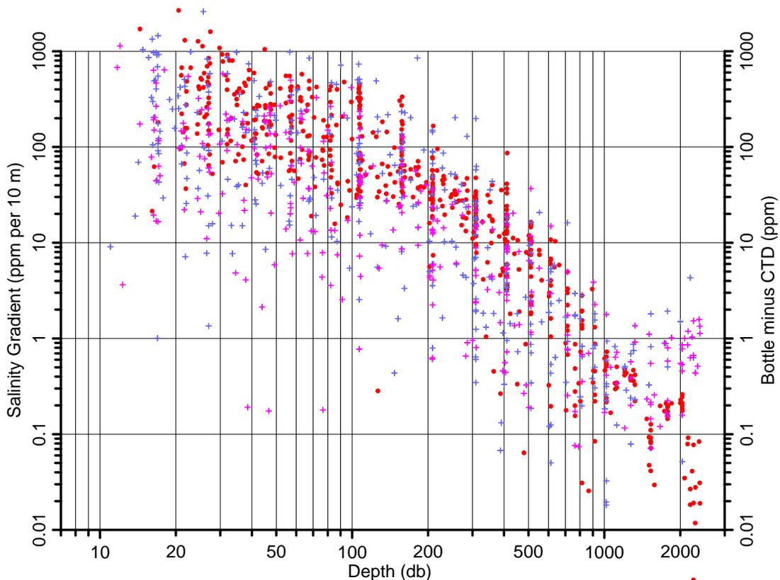
We use data acquired where the salinity gradient is less than 0.001 per metre, typically below 450 m in the region of study. Both TC systems of both SBE9 CTDs indicated salinity too low at 1000 m depth. The calibration data are as follows:
